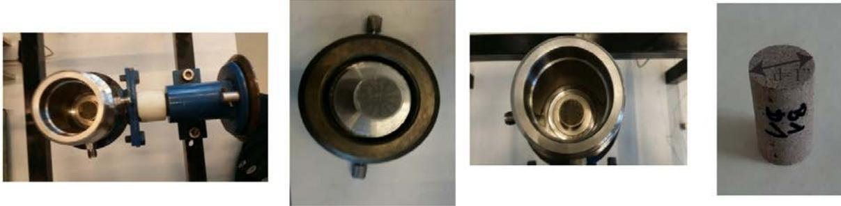
Fig. 9 The experimental cell for permeability tests under various load conditions and the typical sample for the test.
