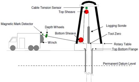
Figure 1 Example of a wireline logging operation. Shown are amongst others, the logging truck with the winch, the drilling rig, the logging sonde (or tool string) as well as the logged borehole .
